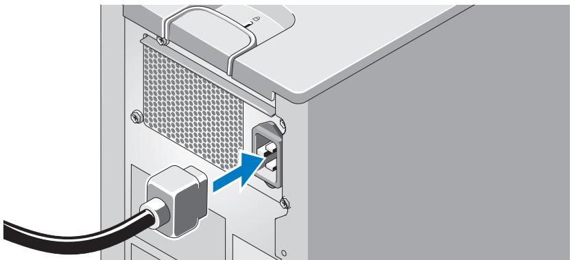
Connect the system's power cable to the system. Next, plug the other end of the power cable into a grounded electrical outlet or a separate power source such as an uninterrupted power supply (UPS) or a power distribution unit (PDU).
